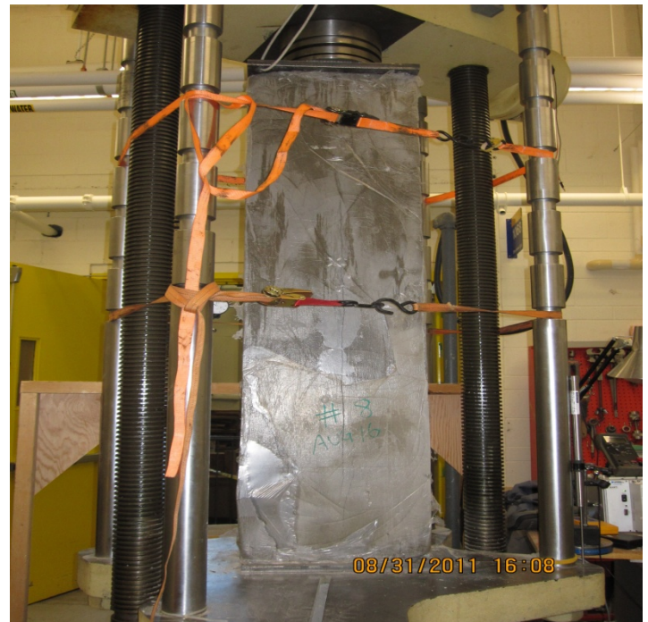
Figure 14. Structural test on a fully instrumented wall constructed with the LGS system and CLC in-fill
