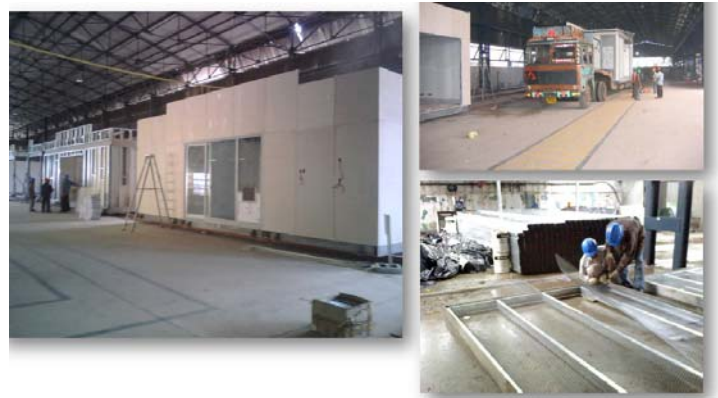
Figure 2. Typical production facility for manufacturing the LGS wall panels in Navi Mumbai (relocated to Bangalore)
